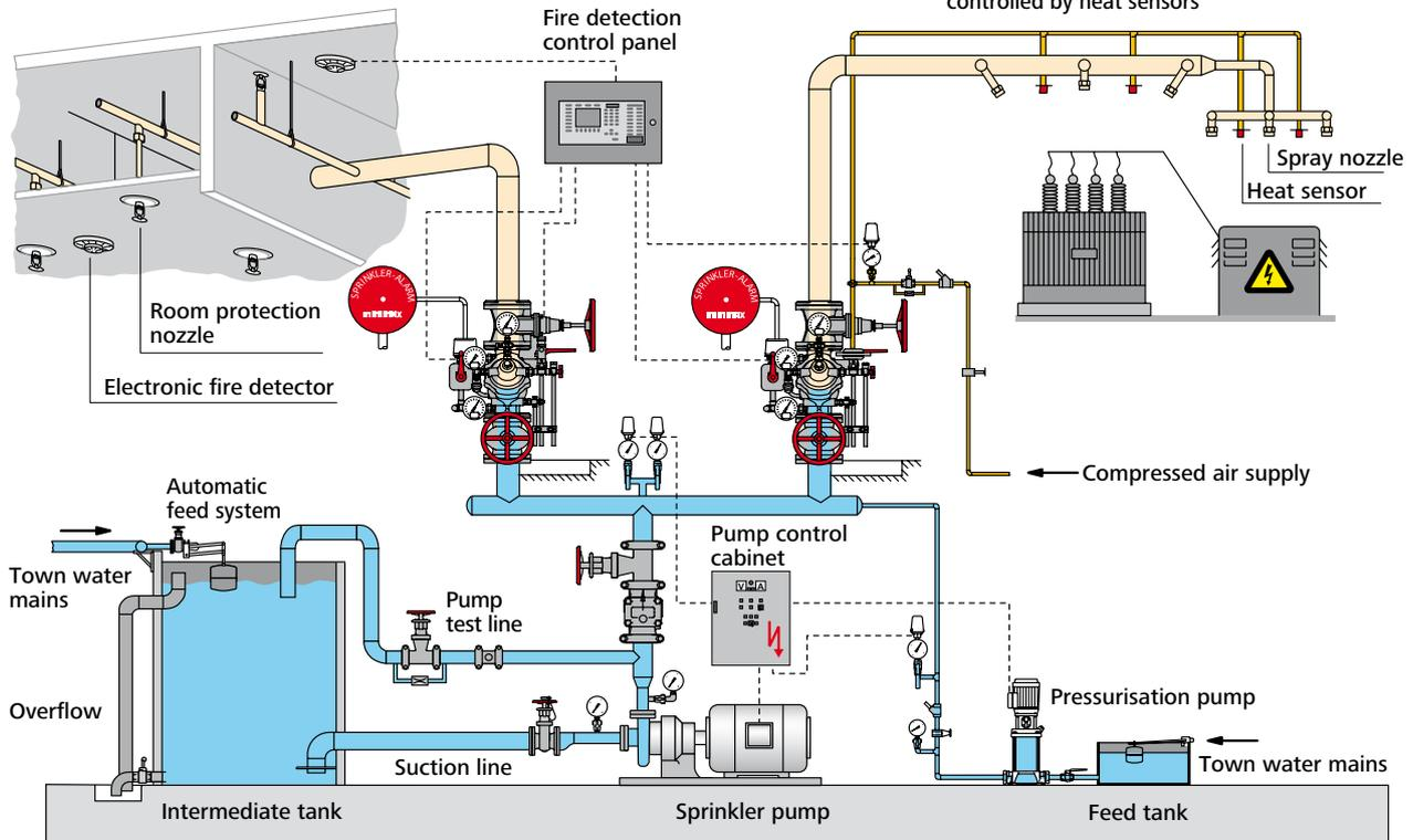
All sections of the building that are to be protected are equipped with a pipe system with open extinguishing nozzles which are divided into several extinguishing areas. In ready mode, all piping up to the deluge valves is filled with water. The system includes fire detectors elements which, depending on the site conditions and the risk, are operated electrically, pneumatically, hydraulically or manually. As soon as a fire is detected, the corresponding deluge valves are
